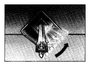
This front view of the SIDE-GUARD stylus protection system demonstrates its operation. The arrow shows the direction the stylus takes when subjected to potentially harmful side thrusts.
